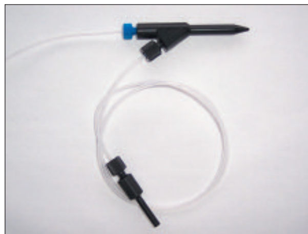
Figure 1: The Burgener Ari Mist parallel path low flow nebuliser.
