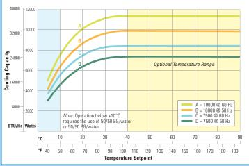
Cooling capacity based on units with P2 pumps with no backpressure. Other pumps will affect cooling capacity performance.
