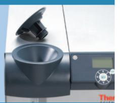
Integrated funnel design allows for spill proof filling.
