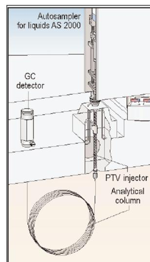
Figure 1: Components of a Programmed Temperature Vaporizing injector instrument
