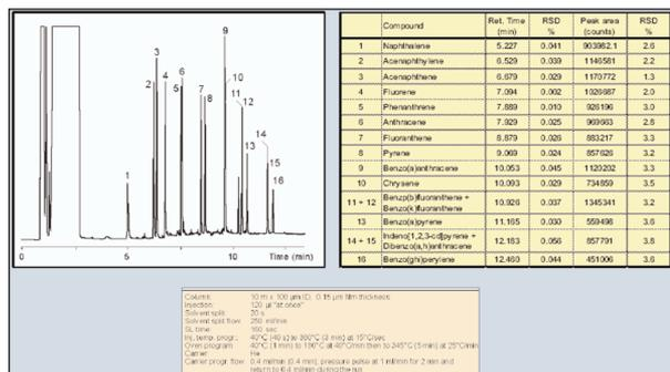
Figure 3: PAHs Analysis by PTV Solvent Split Large Volume Injection concentration in n-pentane 200 ppb
