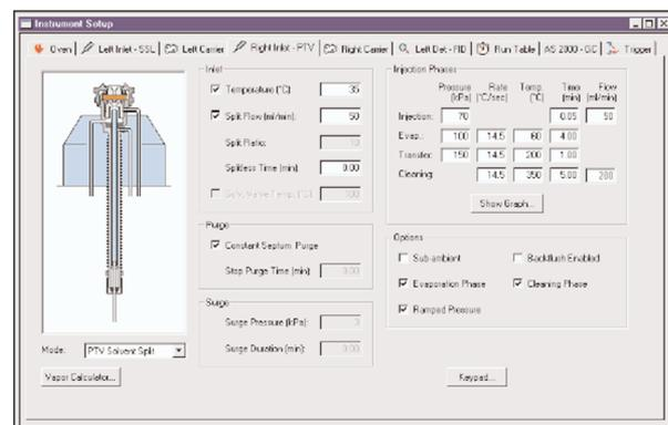
Figure 2: Control parameters for the Programmed Temperature Vaporizing injector
