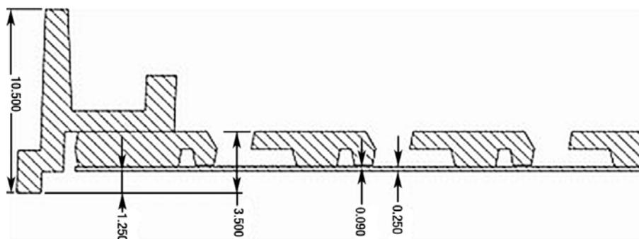
**Figure 4. Top view and cross-sectional side view of the chemotaxis plate with measurements in millimeters.** The height of the gradient region is 90 $\mu$ m. The refractive index of the COP material is 1.53.
