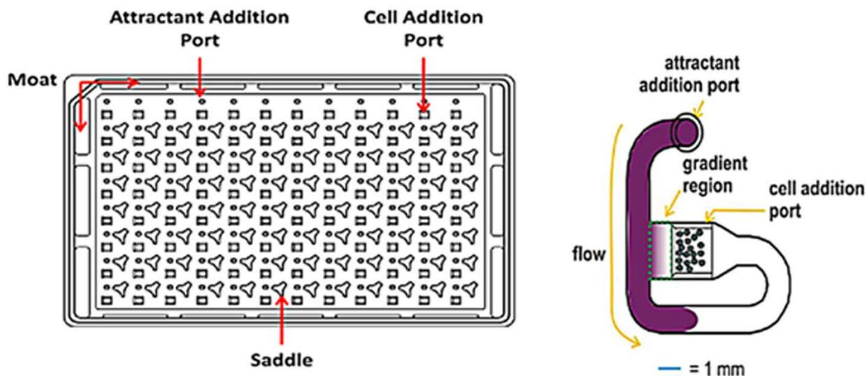
**Figure 2. Overview of the iuvo Chemotaxis Assay Plate and detail of an individual chemotaxis channel.**
