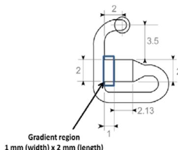
**Figure 5. Gradient region dimensions for imaging.**
