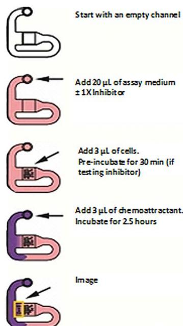
**Figure 1. Schematic of assay protocol using a single plate channel.**
