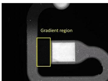
**Figure 8.** Gradient region acquisition using a 1X objective (~90% of the full channel in view) with FITC detection and a 250ms exposure.
