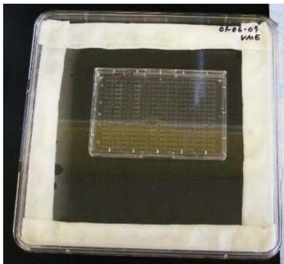
**Figure 3. Lidded secondary container holding the microchannel plate and PBS-saturated towels.**
